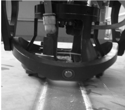
Fig. 13. Photograph of inductor.
